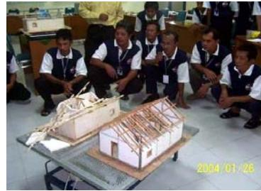
Figure 2: Training mandors (foremen) are watching the different dynamic behavior of non earthquake resistant SEHWM and earthquake resistant SEHWM using various simple demonstration tools, such as small scaled houses on SIMULITAGA SWD-1RM (a simple shaking table)
