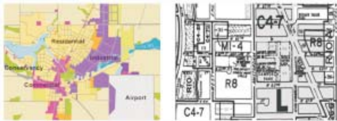
Figure 1. Zoning regulation of New York City contains maps and text that regulate the uses of land and dimensions and placement of structures within various zoning districts. The zoning map shown at left uses district boundaries to separate uses.
